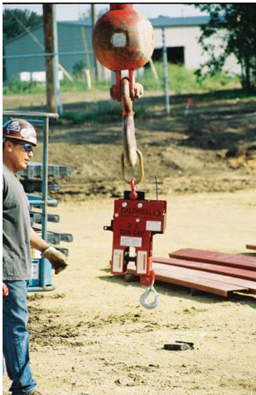
2.5 ton Rig-Release® Hook ready to be rigged
