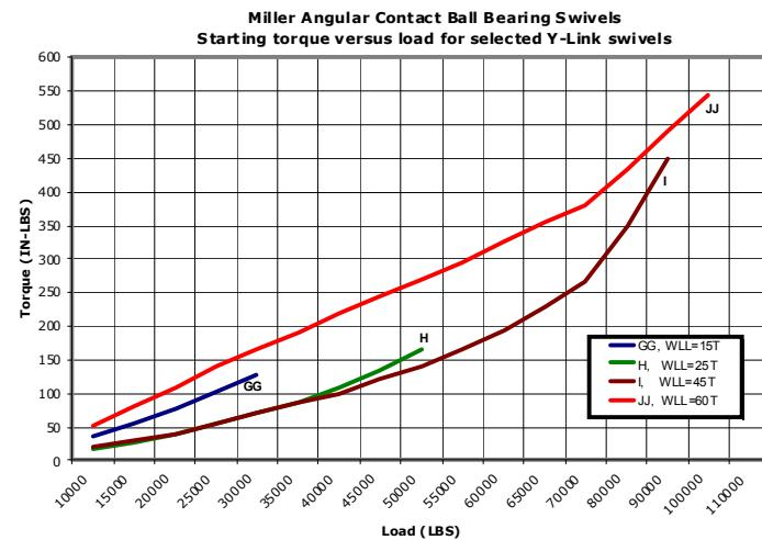
"General guide only, torque value may vary to a significant degree due to application conditions. Miller does not guarantee torque data shown, should specific torque performance be desired, contact Miller"
