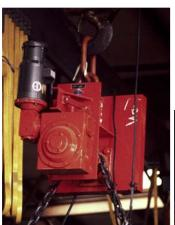
Consists of two powered drive units suspended from two cranes/hoists, with pocketed sheave driving special coil link chain slings that rotate large heavy, bulky items for assembly, welding positioning, and inspection. Drive units can either be operated independently or together, through an operator pendant(s), or remote control.
