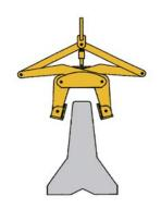
Tong is placed on load in open position. Hoist line must be slack for Auto-Latch to disengage.
