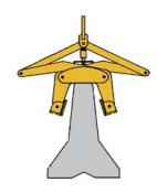
With Auto-Latch engaged, grab is held open to allow removal from the barrier.
