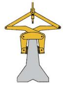
Barrier is placed in position. Hoist line must be slack for Auto-Latch to engage.
