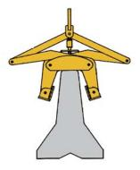
Crane hook is then raised allowing pads to grip barrier.
